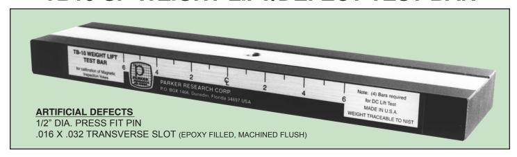
The <u>TB10-SP Magnetic Weight Lift / Defect Test Bar</u> provides for the 10 pound AC weight lift calibration of Magnetic Particle Inspection Yokes, as shown on page 1. Bar weight is certified and traceable to NIST standards. In addition, the reverse side of the TB10-SP bar contains artificial defects as indicated above. Demonstration of actual defect indications is very useful for visual and operational performance purposes.
