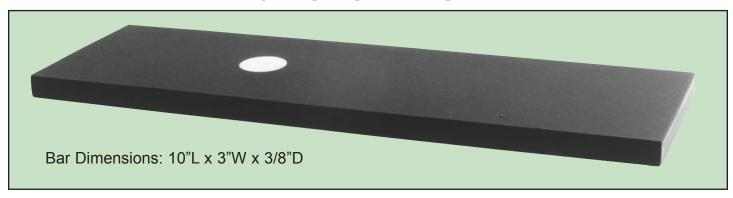
The NA16 Notch Test Bar complies with the requirements of old MIL-STD-271 E and F (Ships) paragraph 4.3.1.2 and NAVSEA-TB-T9074-AS-GIB-101-271. The requirement reads as follows:
