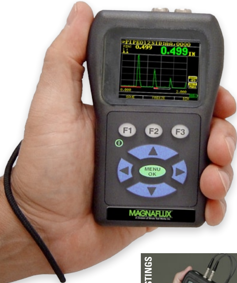
◀ The Magnaflux MT-2100 (color display) displaying echo to echo fully rectified
